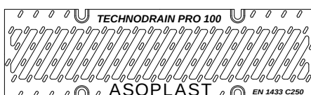
7 DUCTILE IRON GRATING C250 SLOT 10 mm
