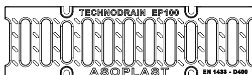
① DUCTILE IRON GRATING D400 SLOT 18 mm
